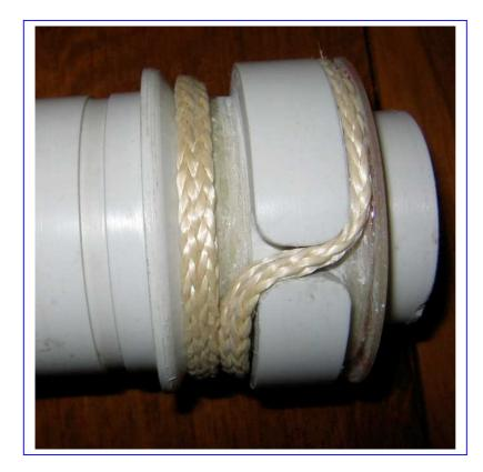
The photo to the left shows the Vectran coming from aft, passing through the drive groove, and then proceeding around the front of the boss in the retaining groove whereupon it will exit aft through the other drive groove.
